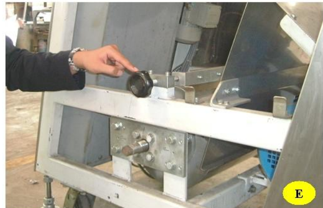
Step 4: Loosen the bigger size flower knob at the bottom until there is a gap / space / distance between the flower knob and the inner bottom shaft.
