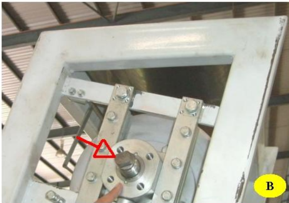
Step 2: Loosen the screw shaft (pic. B) on top of machine until there is a space / gap / distance between screw shaft and the top drum (pic. C).
