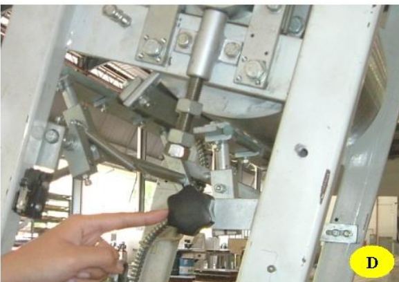
Step 3: Loosen the medium size flower knob on the top until there is a gap / space / distance between the knob and the inner shaft.
